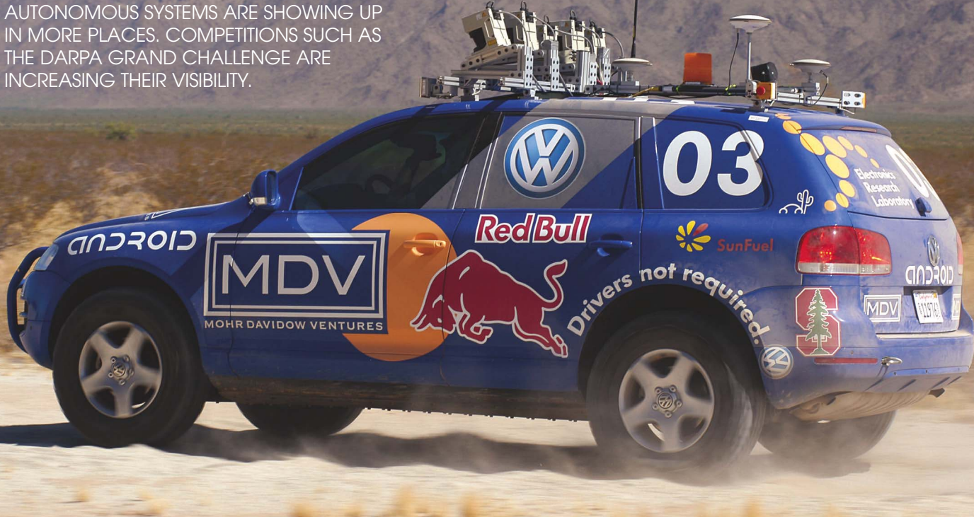
Figure 1 Stanford Racing Team's autonomous vehicle, “Stanley”—a reinforced Volkswagen Touareg with a custom drive-by-wire system, a sensor rack, and a computing system—won the 2005 DARPA Grand Challenge (courtesy Stanford Racing Team).
